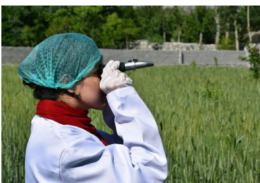
Rozina using a refractometer to check solid sugar content from a sample of freshly harvested honey.
