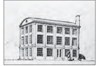
Fig. 8: İstanbul, reconstructed image of a prefabricated cast and wrought-iron corn mill erected by the Scottish shipbuilder William Fairbairn in 1840.
