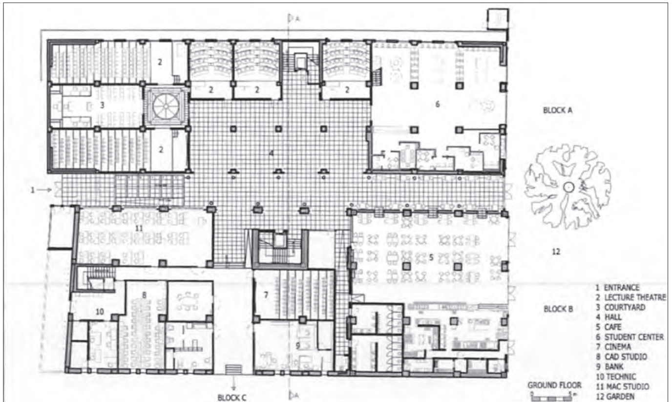
Fig. 24: BU Campus, ground floor plan of the two buildings after their integration into a unified complex.
