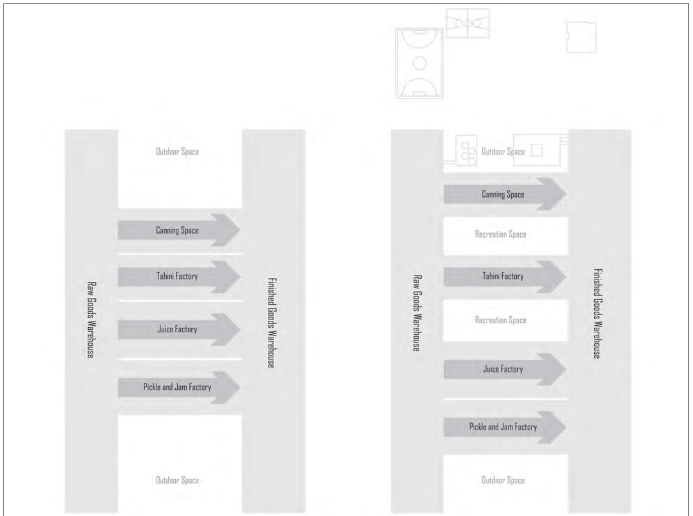
Fig. 12: Bekaa Valley, Lebanon, Food Canning Factory, Hashim Sarkis, Architecture, Landscape, and Urban Design, 2003 (on hold); ladder diagrams showing the path of goods in the production process.
