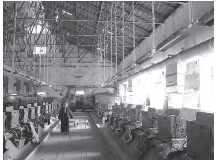
Fig. 29: Damanhur, Abdel-Meguid Barakat Ginning Mill, early-20 th century; interior view showing the original wooden floor and roller gins of the mill, which is still in use.
