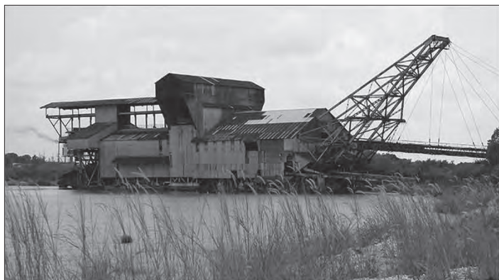
Fig. 1: This 4,500-ton giant tin dredge started operation in 1938 and is the last to survive of 352 dredges that had functioned in Malaysia. It once belonged to the Southern Malayan Tin Dredging company, but is now only a reminder of a time when Malaysia was the world's greatest tin producer.
