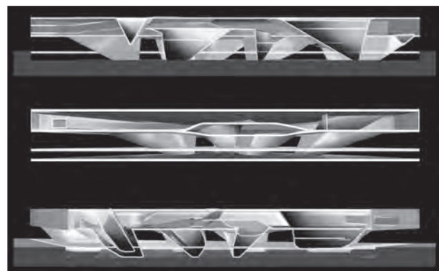
Fig. 5b: Wolfsburg, Germany, Phaeno Science Centre, Zaha Hadid Architects (structural engineers: Adams Kara Taylor), 2005; this project provides a form where conventional walls, floors, and columns merge to produce a single surface with 'morphed fluid geometries' that are difficult to define as conventional platonic shapes.
