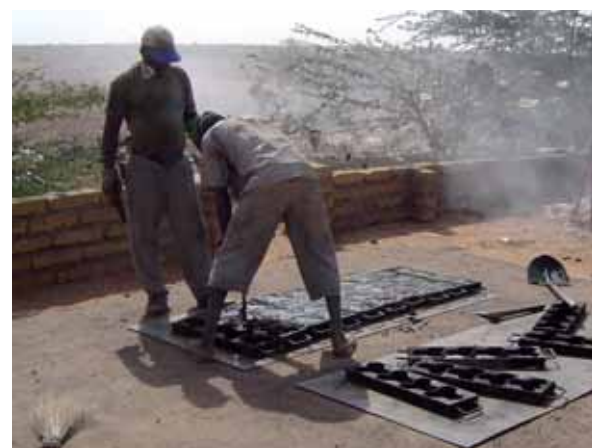
Plastic material is melted and mixed with river sand and compressed in moulds to produce solid pavement bricks.
