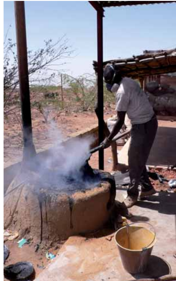
Plastic material is melted and mixed with river sand and compressed in moulds to produce solid pavement bricks.
